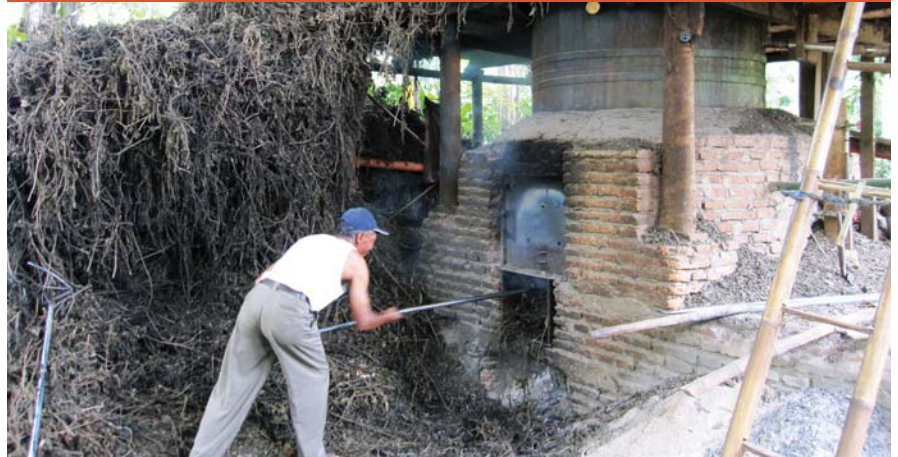
Eco-friendly traditional patchouli distillation using patchouli waste as firewood in East Java
