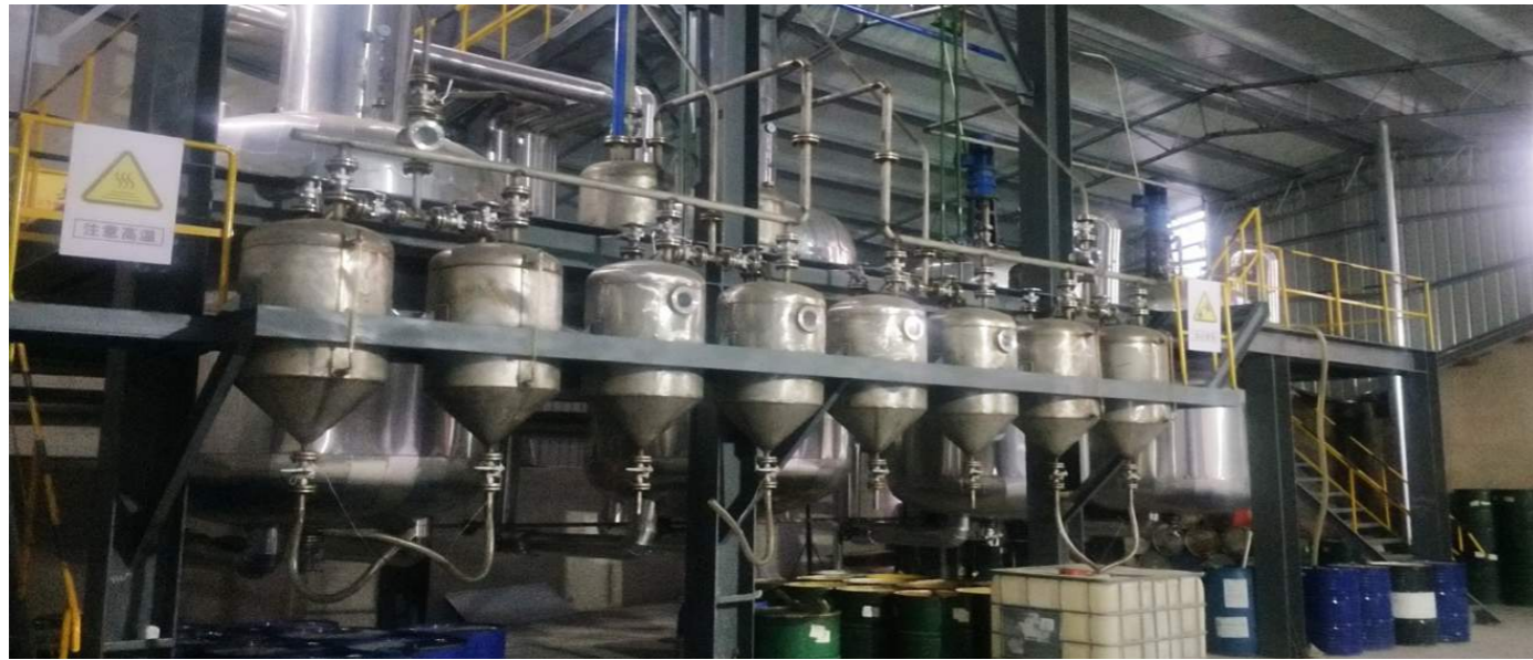
SEPARATING CEDRENE AND CEDROL FROM THE CRUDE OIL
